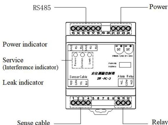
◆ Install the detector in a secure indoor collection box or cabinet where it is easy to maintain and check. Avoid high temperature, high humidity, vibration, corrosive gases, and other electronic interference sources. XW-PC-3A sensor buckle is mounted on a standard 35 mm DIN rail.
