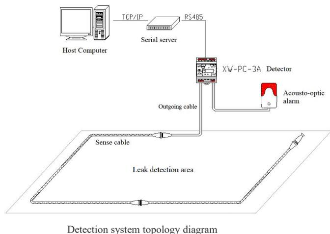
XW-PC-3A sensor connect with sense cables, and once the liquid is detected, the leakage data can be uploaded leakage data to the host computer through RS485 signal, accurately locate the leakage position and trigger the relay action. Sensor relay output signal can be used to control peripheral equipment such as acousto-optic alarm, automatic valve and intelligent alarm, etc.
