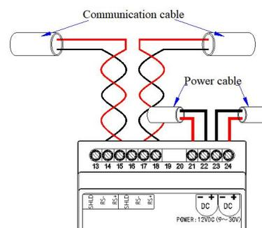
**Connect power cables and communications cables**
